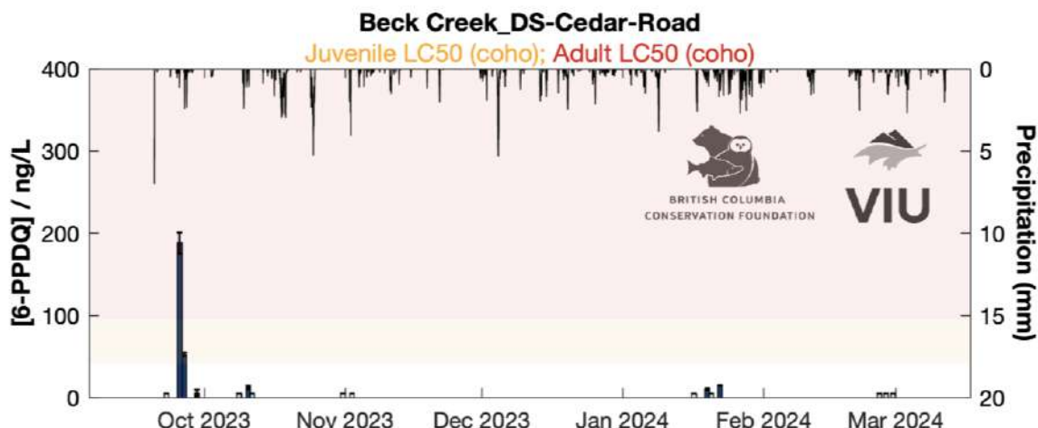
Figure 13. Sample results from samples collected at the Beck Creek site located downstream of Cedar Road between late September 2023 and March 2024. The 6-PPDQ concentration is expressed along the left axis, while the precipitation from the nearest weather station is found on the right axis and runs opposite (top down). Empty bars (black outline, no fill) represent a grab sample that was analyzed, but no 6-PPDQ was detected. The yellow shaded portion of the graph, beginning at 41 ng/L, represents the currently accepted LC 50 of juvenile (alevin) coho salmon. The red shaded area of the graph, beginning at 95 ng/L, represents the currently accepted LC 50 of smolt and adult coho salmon.
