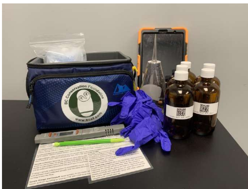
Figure 7. An example of the wide scale surveillance grab sampling kit that was provided to each of the participating groups. Kits were scaled up or down depending on the number of sample locations the group was monitoring.
